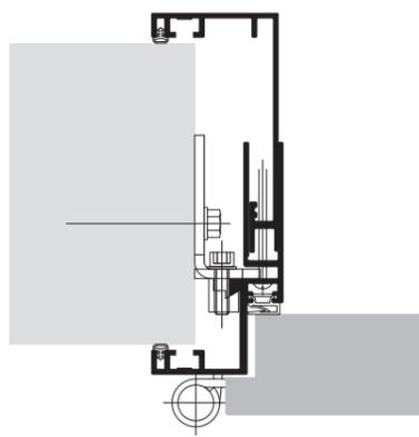
Aluminium frame type Hardline for dulled doors
