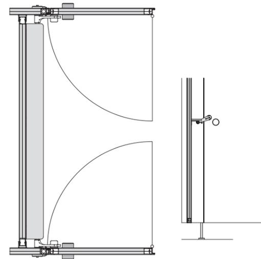
Synchronous locking of the changing cubicle with central lever locking.
