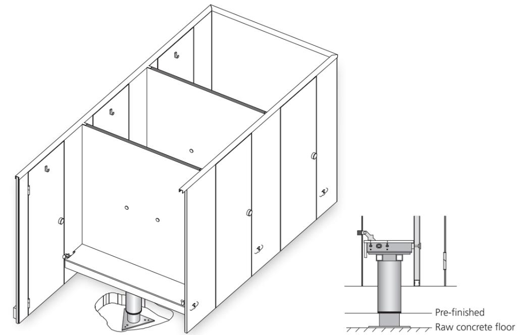
The optional central midfoot under the cubicle bench is anchored to the raw concrete floor. This means that the entire cubicle can be supported on one foot and feet in the front are largely unnecessary.
